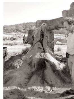
View of the borehole used by the Kestanbol spa. The tubes are hidden by thick travertine deposits produced by the leaks of thermal brine water. The colour is due to iron precipitations.
