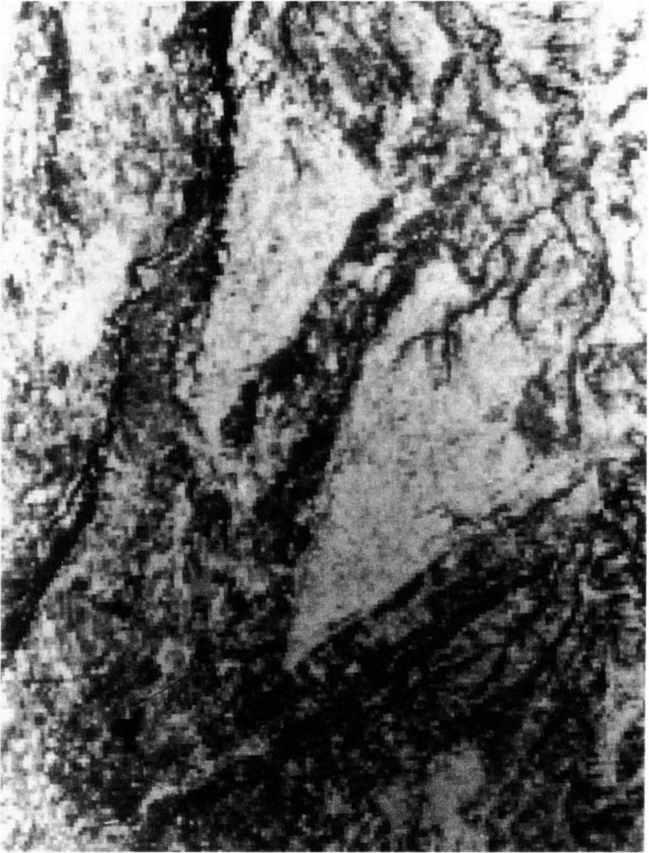
Figure 14. LANDSAT 5 thermal infrared band. Light gray zones = sand and gravel terraces (greater depth to water); dark gray = earlier alluvial valley floors (lower depth to water); black = shallow groundwater and discharge to stream network.
