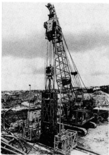
Figure 25: Overall view of the horizontal multi-axis rotary excavator.
