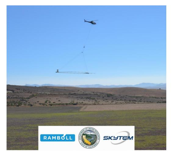
The SkyTEM airborne electromagnetic system is suspended approximately 100 feet above the ground surface from a Sinton Helicopter that flies about 50 mile per hours. The output data provide electrical resistivity values for the underlying geology, which translate into texture profiles of sediments comprising aquifer systems. For more information on California's AEM Project visit **DWR-AEM**
