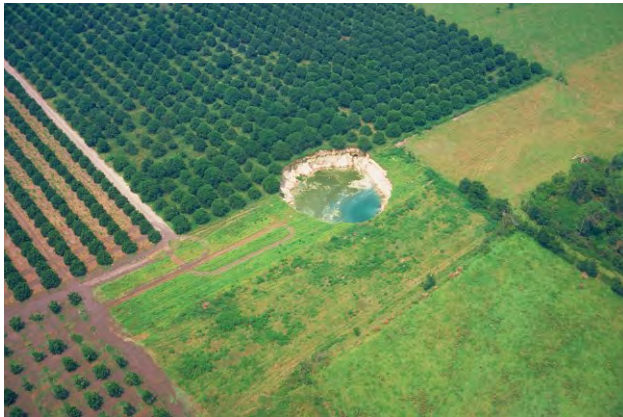
Figure 3.6 New sinkholes frequently open in Florida, often triggered by anthropogenic factors such as groundwater pumping for irrigation ( photo on the left ) and water supply, modified surface drainage controls, failing/leaky water and sewer pipelines, mining, and other activities which interrupt a delicate balance between the surficial and Upper Floridan aquifers separated by a thin confining layer. Right : The infamous Winter Park sinkhole that suddenly opened in 1981, causing serious damage. Both photos by Professor George Sowers, courtesy of Francis Sowers.
