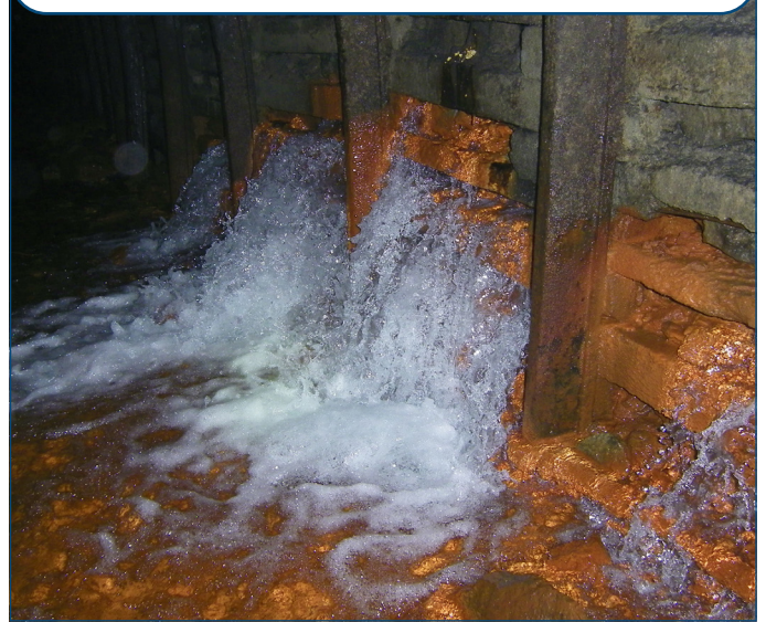
POMORZANY — POLAND GROUNDWATER INFLOW TO ZINC & LEAD ORE MINE
